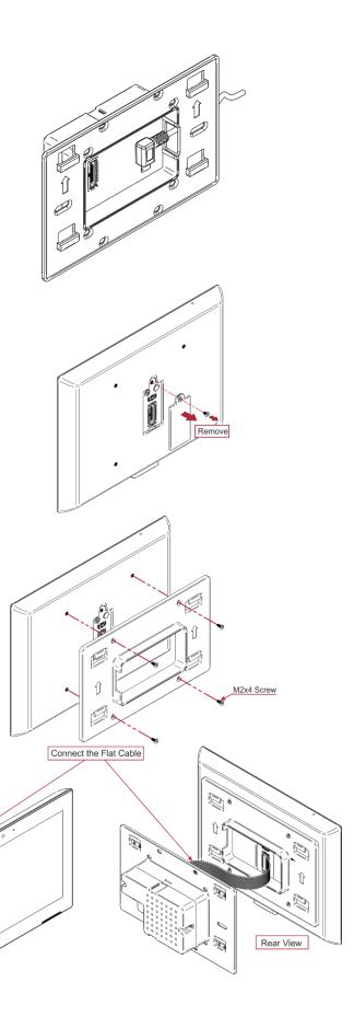
5. Slide the Touch Panel panel-mount tabs over the grooves on the on-wall mount unit.
