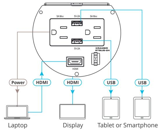
Figure 3: Connecting RTBUS-24
