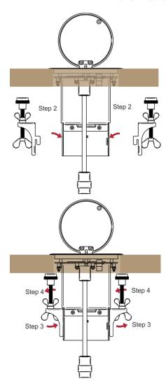
**Step 3**: Tighten the butterfly mounting screws securely upward against the table.
