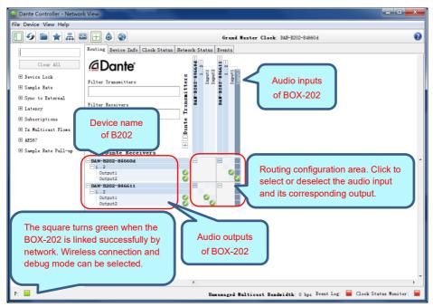
The default setting only supports 2 transmit and 2 receive flows, if more than 2 devices are needed, please click any device to enter **Device View** page.
